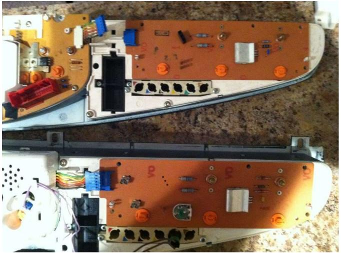
The wiring portion is very simple. The S4 has a two pin harness that plugs into the cluster. The S6 only has a single pin. If you have acess to a parts car you can clip and swap harnesses. For a cleaner install you could repin the S6 harness with an additional pin and run your new lead. Run a wire however you would like to route it. I ran it along the factory cluster harness, down into the drivers kick and through the gromet in the firewall that holds many other wires/cables.
