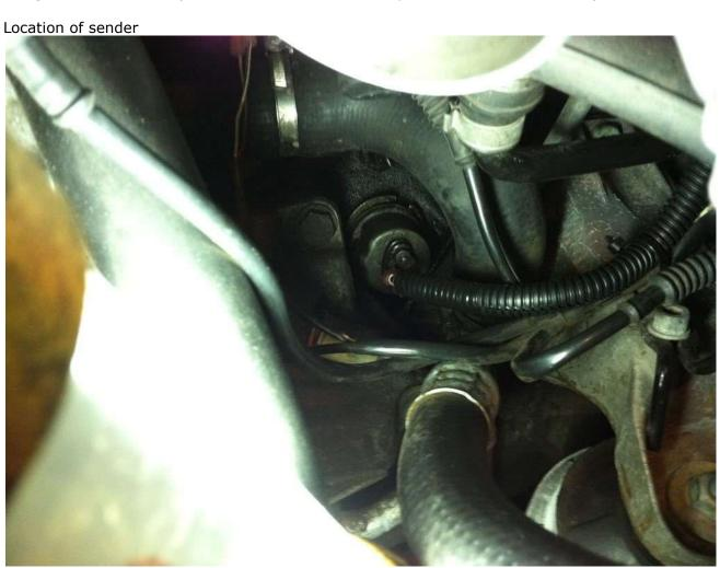
Attach an end to the wire, slip it on the sender. Zip tie up any loose wire in the bay and reinstall cluster with newly pinned harness. You should now have an active oil pressure gauge in place of your old volt gauge.
