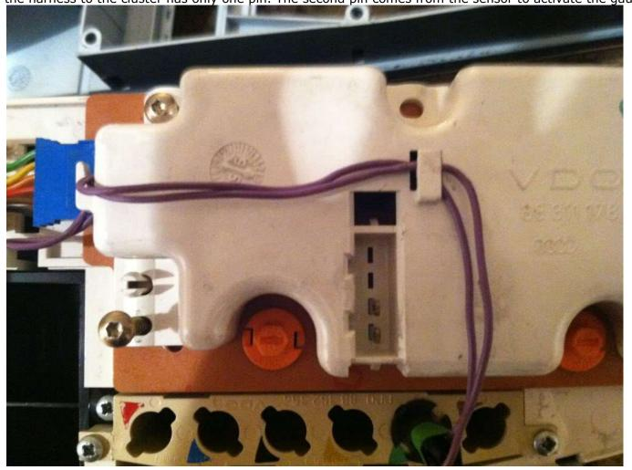
Install the gauges on the S4 circuit board and install them into the S6 cluster as they were. \*NOTE\* the clock was also different on mine. This could probably be resolved if you are circuit board savy, I just swapped clocks as well.
